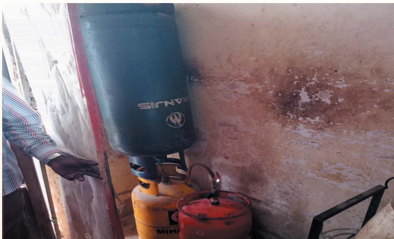
Figure 31: 38kg gas cylinders from Manjis being decanted to 6kg gas cylinders from Lake and Oryx
