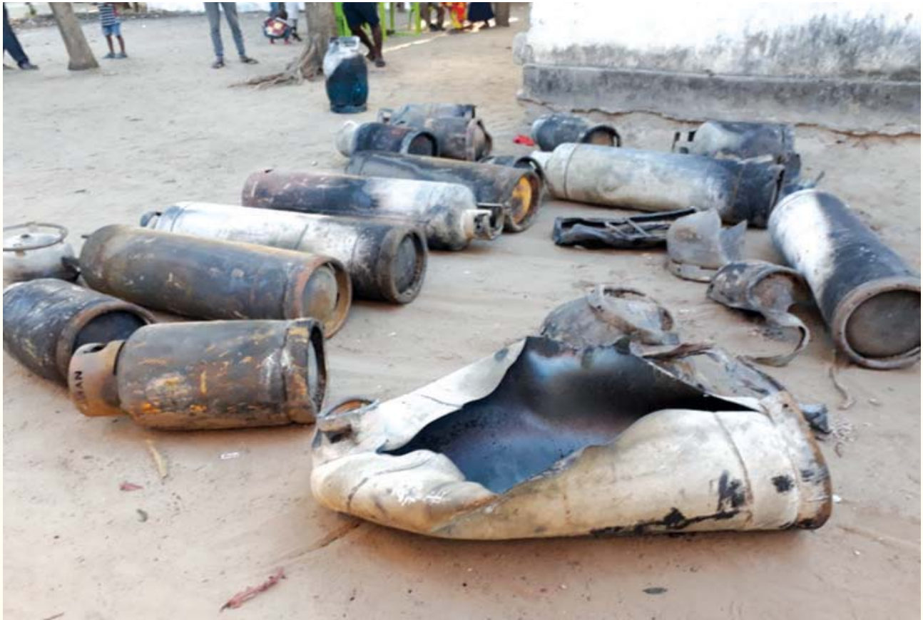
Figure 34: Exploded and burnt LPG cylinders at Kwa Mapunda area, Chamazi ward in Temeke, Dar es Salaam
