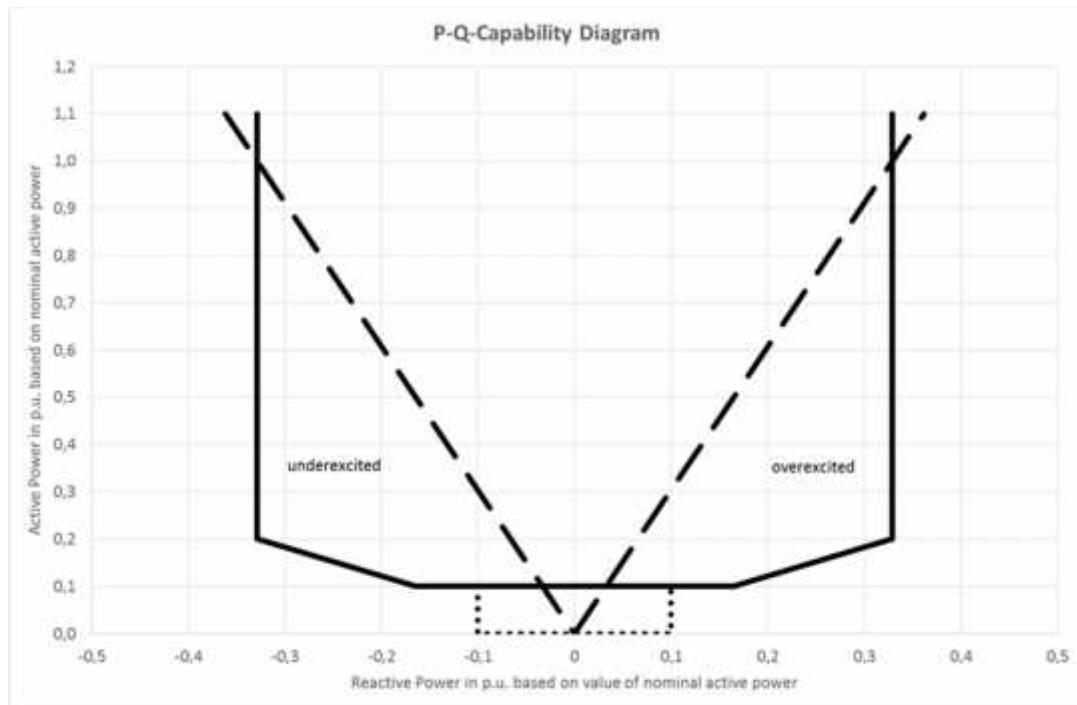
**Figure 3.1:** P-Q-Capability Diagram (generation oriented),
